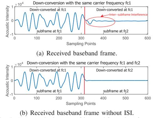
Fig. 5. Remove the impacts of inter-subframe interference.
